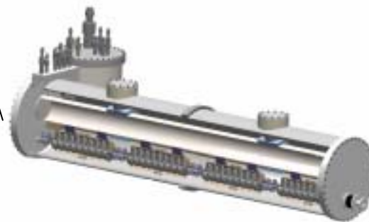
Cryomodule 4 x 9-cell cavities
