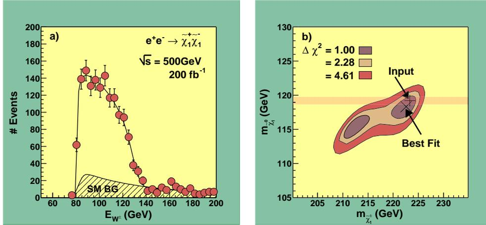
**Figure 2.11:** (a) Energy distribution of the final-state  $W^\pm$  from chargino decays:  $\tilde{\chi}_1^\pm \rightarrow W^\pm \tilde{\chi}_1^0$  (points with error bars) after the acoplanarity angle cut at  $\theta_A = 30^\circ$ . The solid curve is the best-fit curve to determine  $m_{\tilde{\chi}_1^\pm}$  and  $m_{\tilde{\chi}_1^0}$ . (b) Resultant contours from the 2-parameter fit.
