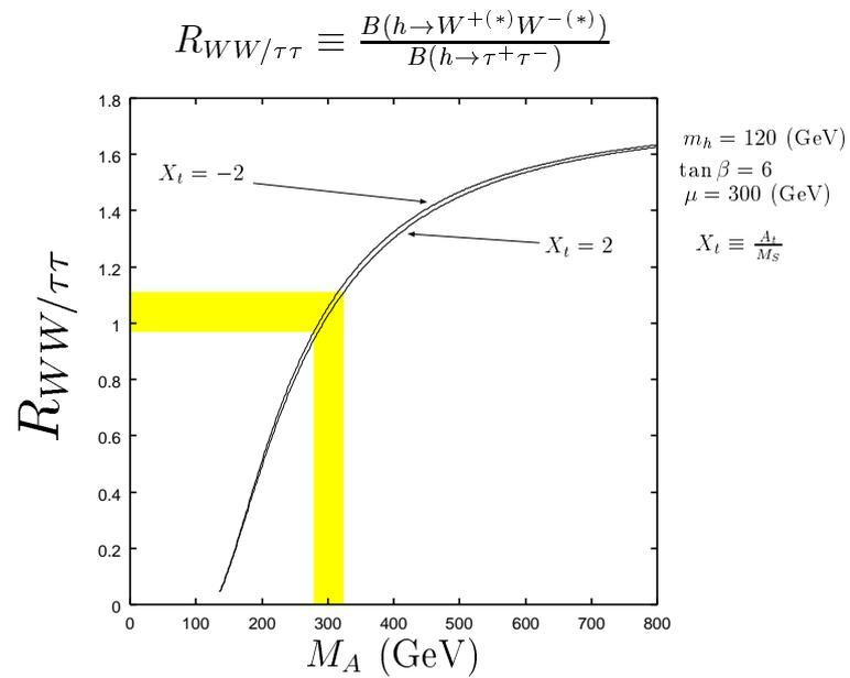
**Figure 2.6:** Ratio  $B(h \rightarrow W^{(*)}W^{(*)})/B(h \rightarrow \tau^+\tau^-)$  for the 120 GeV lightest Higgs boson for  $\tan\beta = 6$ ,  $\mu = 300$  GeV and  $X_t = \pm 2$  as a function of  $M_A$ . The shaded area shows the  $M_A$  determination from this ratio, obtained by assuming that  $B(h \rightarrow W^{(*)}W^{(*)})/B(h \rightarrow \tau^+\tau^-)$  is determined with 6.7% accuracy.
