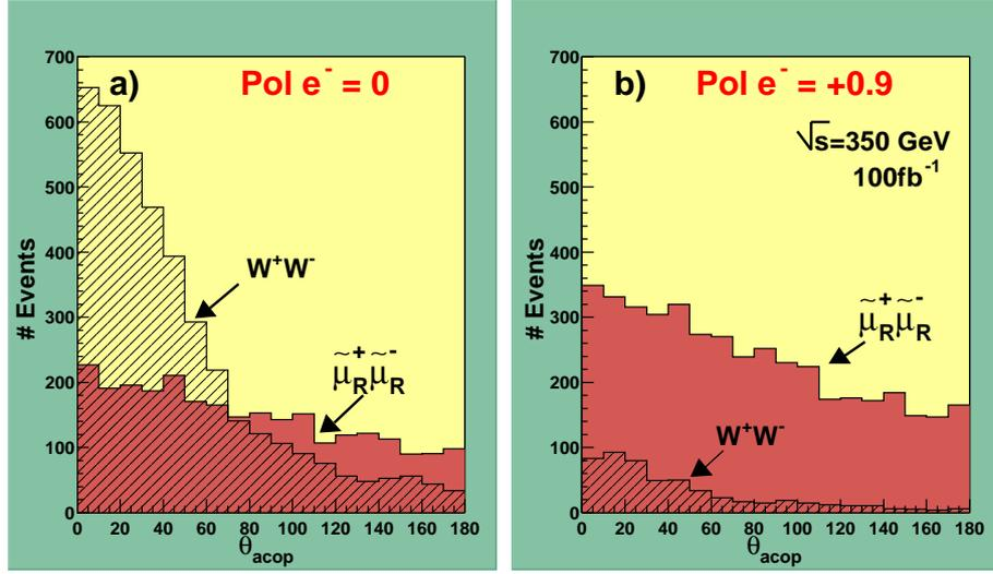
**Figure 2.8:** Examples of acoplanarity distributions for smuon pair productions. The Monte Carlo data correspond to an integrated luminosity of  $100 \text{ fb}^{-1}$  at  $\sqrt{s} = 350 \text{ GeV}$  with (a) an unpolarized electron beam and (b) the right-handed electron beam. The solid histograms are for the signal events, while the hatched histograms are the background from  $W^+W^-$  production.
