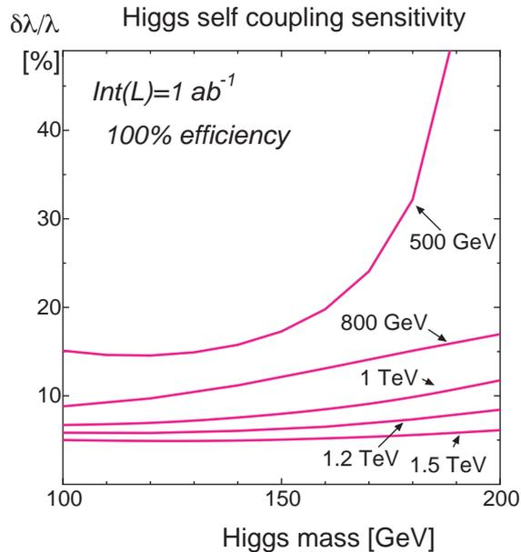
**Figure 2.5:** Accuracy of the triple Higgs boson coupling measurement at GLC based on the production processes of  $e^+e^- \rightarrow ZHH$  and  $e^+e^- \rightarrow \nu\bar{\nu}HH$ . The integrated luminosity is assumed to be  $1000 \text{ fb}^{-1}$ , and 100% electron polarization is assumed for  $e^+e^- \rightarrow \nu\bar{\nu}HH$ . The efficiency correction is not included.
