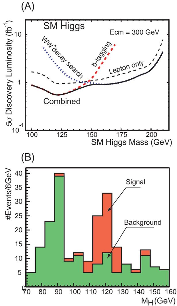
**Figure 2.1:** (A) Integrated luminosity required for a  $5\sigma$  discovery of the Standard Model Higgs boson. (B) Invariant-mass distribution for the Higgs boson search at GLC with an integrated luminosity of  $5 \text{ fb}^{-1}$  at  $\sqrt{s} = 300 \text{ GeV}$ . Signals for the Standard Model Higgs boson of  $120 \text{ GeV}$  and backgrounds are shown in red and green, respectively, for combinations of the 4-jet, 2-jet + missing, and a lepton pair +  $b\bar{b}$  modes.
