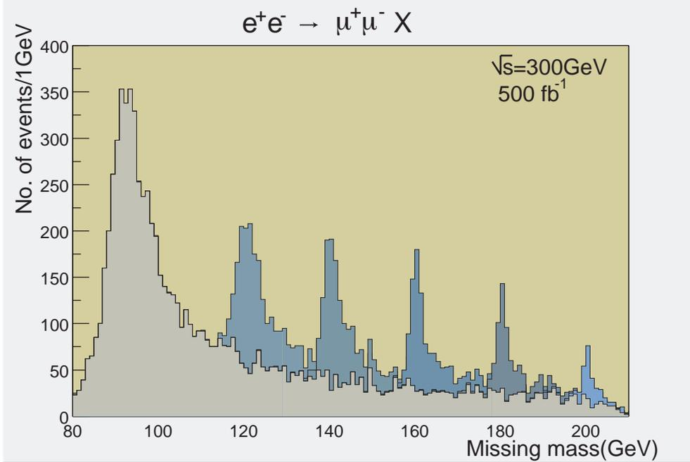
**Figure 2.2:** Distribution of the recoil mass of the  $\mu^+\mu^-$  pair in  $e^+e^- \rightarrow \mu^+\mu^- X$ , normalized to  $500 \text{ fb}^{-1}$  at  $\sqrt{s} = 300 \text{ GeV}$ . The background from the  $Z^0$ -pair production process,  $e^+e^- \rightarrow Z^0Z^0, Z^0 \rightarrow \mu^+\mu^-$ , and the SM Higgs boson signals with masses set to 120, 140, 160, 180 and 200 GeV are shown.
