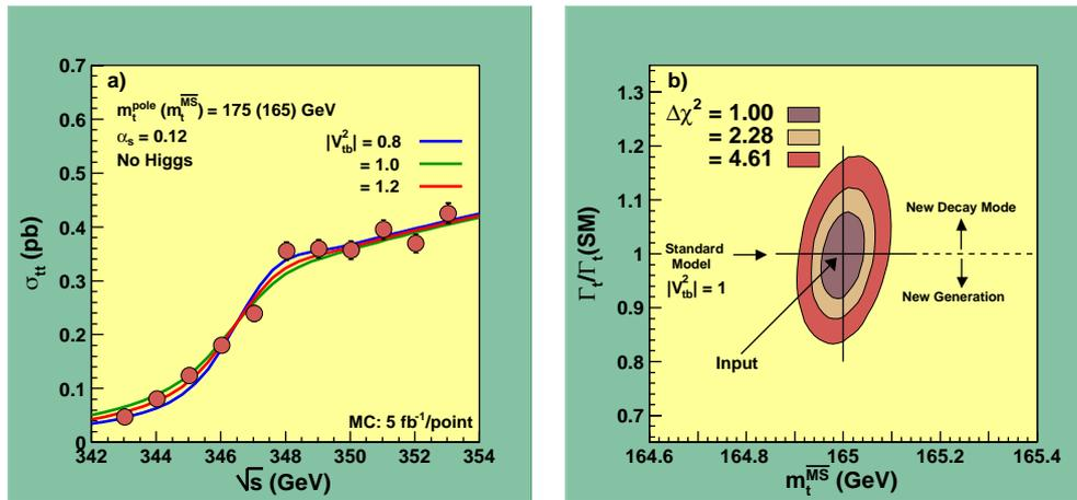
**Figure 2.15:** a) Dependence of the cross section on  $\Gamma_t \propto |V_{tb}|^2$ . A sample simulation of the energy scan is superimposed, where each point corresponds to data collected with an integrated luminosity of 5 fb<sup>-1</sup>. b) The contours obtained from the fit to the data points.
