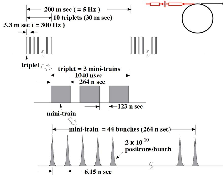
Figure 2: Timing structure in the positron source.
