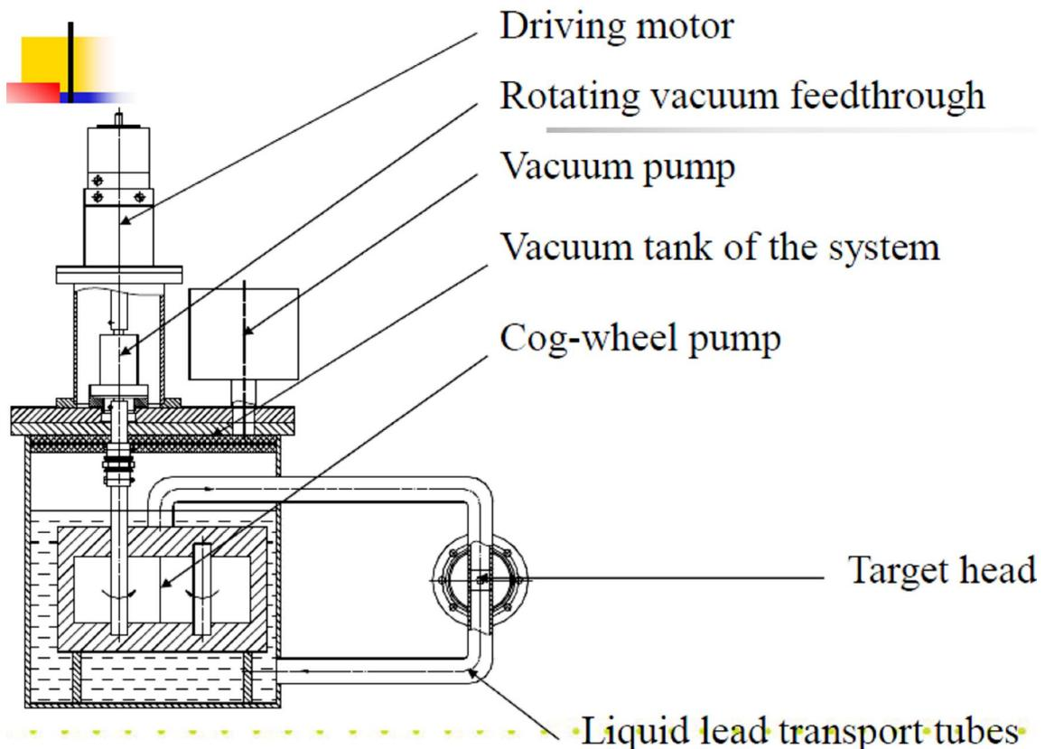
Fig.1 The prototype of liquid lead positron production target which is under commissioning with 50kW electron beam.
