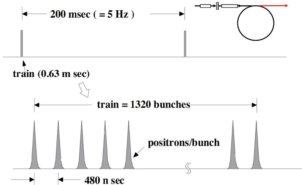
Figure 3: Timing structure in the positron source.
